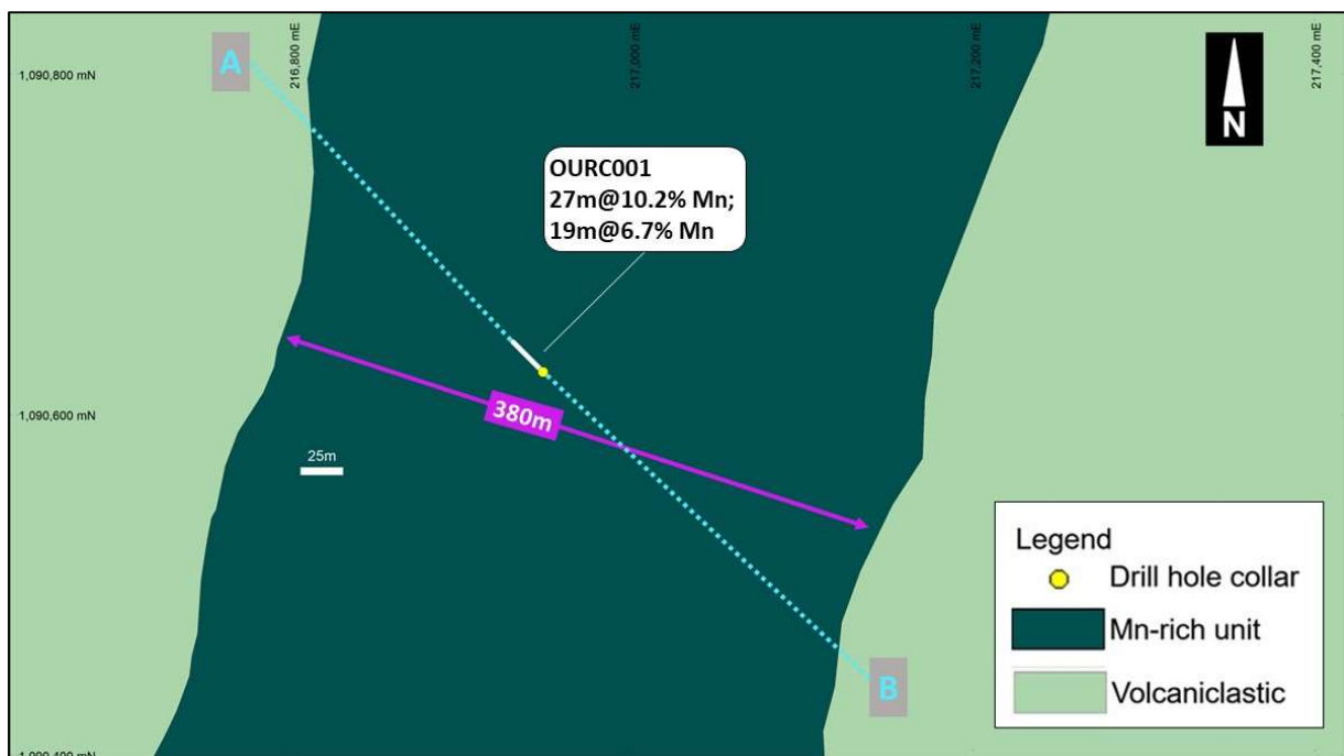
Figure 4 Drill hole OURC001 which intersected 46 metres of manganese – section line shown in blue
